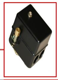
The LF17 pressure switches are used to regulate the tank pressure between two preset values on small electrically driven air compressors (up to 175 psig). They are available with an unloader valve, which prevents compressors from starting under load. This is a heavy duty unloader switch.
